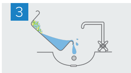
3 When the basin is emptied, microorganisms can be retained within the basin.
