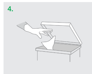
4. Change the wipe if it becomes dry or soiled and discard. Ensure that the surface remains wet for a minimum of one minute.
