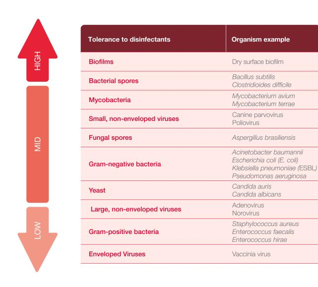
Typical tolerance of microorganism types to disinfectants, adapted from McDonnell & Russell<sup>8</sup>
